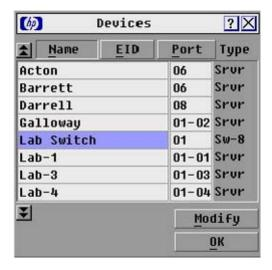
When the HP KVM Server Console Switch G2 discovers a cascaded HP KVM Server Console Switch G2, the port numbering changes automatically to accommodate each server. For example, if the HP KVM Server Console Switch G2 is connected to port 02, the switch port is listed as 02, and each server under it is numbered sequentially 02-01, 02-02, and so on.
